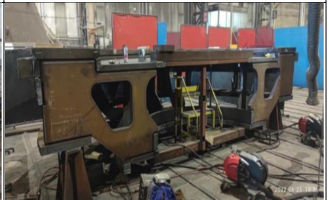
EM-01_U3# Headcover Fitting in process in China
