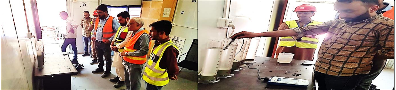
The JAR test conducted for the waste water of Tholki crusher plant at CGGC Laboratory Barseen
